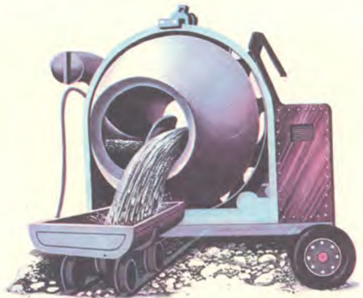
CEMENT MIXER The round bowl part of this machine mixes sand, water and powdered cement into the substance used for building.
