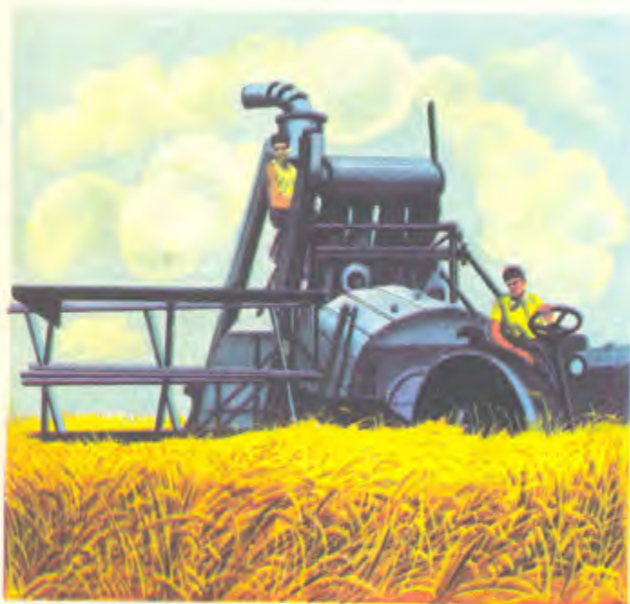
COMBINED HARVESTER This machine reaps and threshes corn or wheat at the same time.
